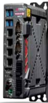
The **MC6N-ECAT** is a high performance Motion Coordinator dedicated to running remote servo and stepper drives via EtherCAT. It is based on the 1GHz i.MX7 Dual ARM Cortex A7 Core Processor supporting up to 64 axes of motion for ultra precise axis resolution.
