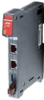
**Flex-7** is an advanced motion controller supporting up to 128 axes with multi-tasking capability via EtherCAT, with update rates down to 125µs. Flex-7 has separate cores dedicated to motion and communications combined with Gigabit Ethernet.
